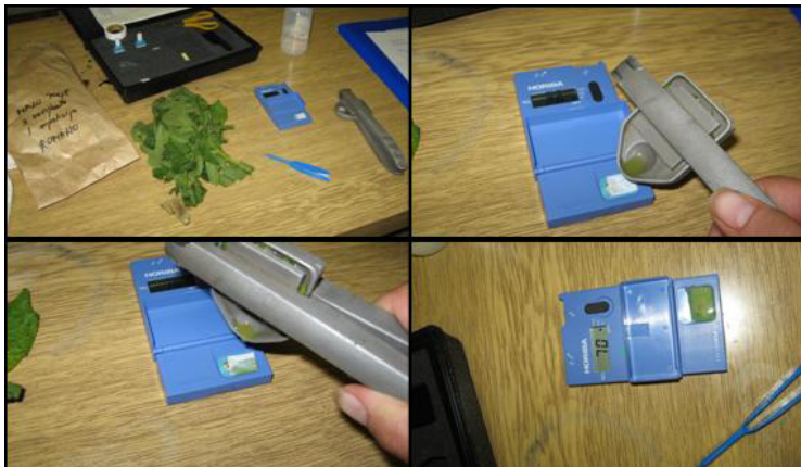
Fig. 2. Measurements of \text{NO}_3 -N from petiole sap of potato crop by Cardy ion meter.
